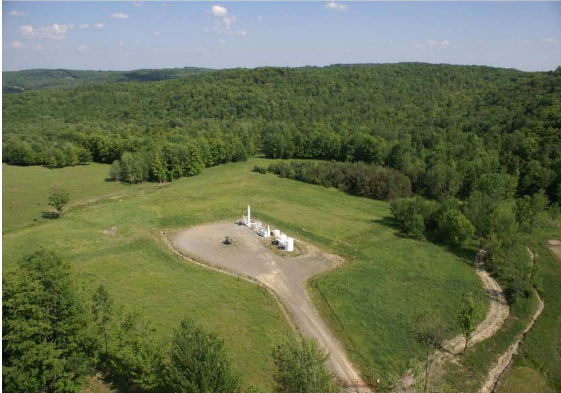
Figure B8.7 A well pad in production in the NE United States 13
