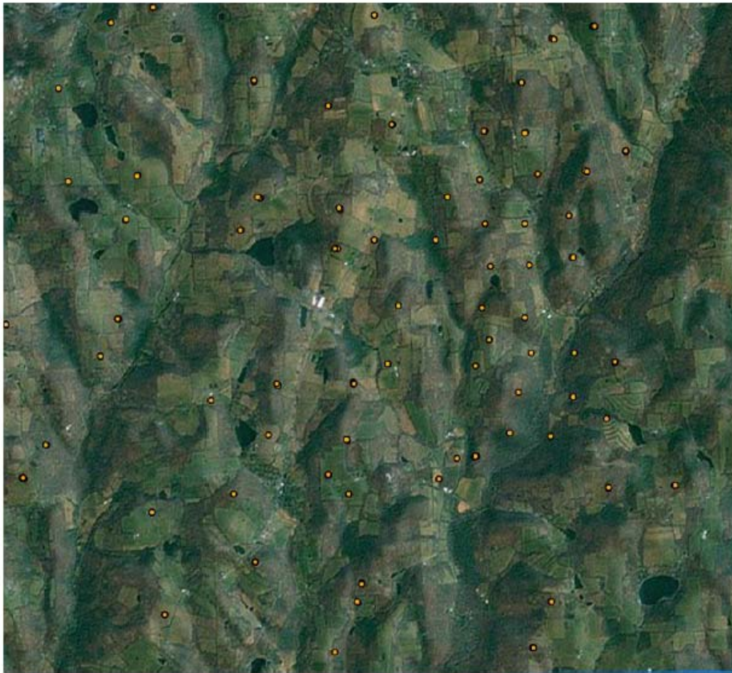
Figure B8.6 A local network of shale gas wells in the NE United States (57 wells covering 90sqkm) 11
