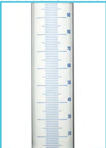
This is an up close view of the measurements on a graduated cylinder. (The term “graduated” refers to the unit markings as they go up, or “graduate,” in scale.)
