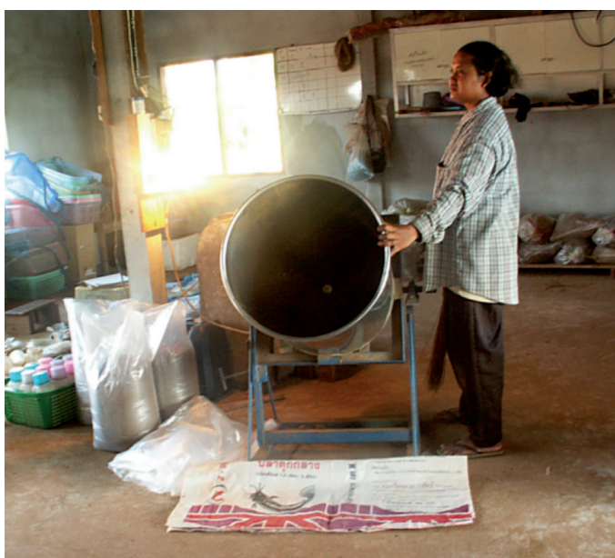
FIGURE 4 Locally designed feed mixer with 15 kg capacity for sex-reversal feed production
