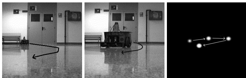
Figure 5: Beginning (left) and end (center) of a moving robot path. In the right picture we display the results provided by the detector in four discrete instants of time; the dot size means proximity to robot camera. The arrows are only a guide to the eye.
