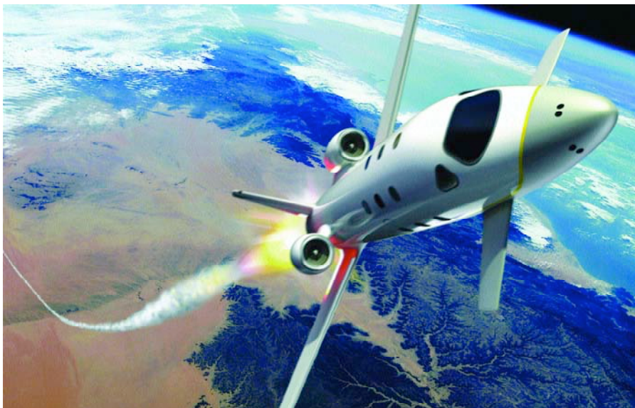
Subordinal Flight is an EADS Astrium concept for a takeoff and one-stage journey into space for up to five people. Beginning with a 45-minute cruise to an altitude of 12 km, rocket propulsion takes over from the jet engines and the space plane is boosted in almost vertical attitude for 80 seconds to ascend to over 100 km (EADS)
