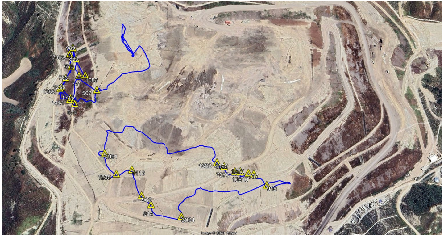
FIGURE 2: IRWIN 439: SURFACE EMISSIONS MONITORING PATH WITH MONITORED EXCEEDANCE CONCENTRATIONS, 1/9/24
