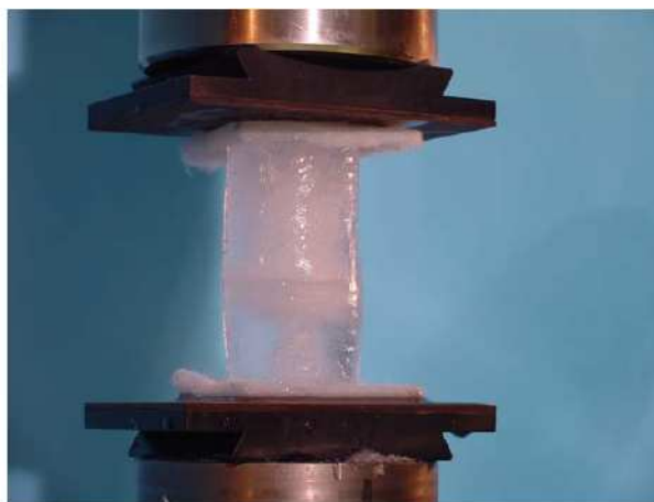
Figure 8.16 Mounted ice cylinder test specimen
