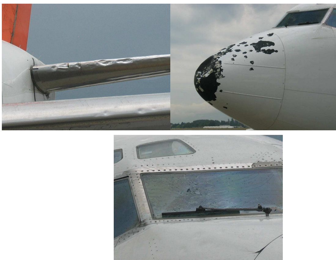
Figure 8.39 Hail damage to Boeing 737 aircraft
