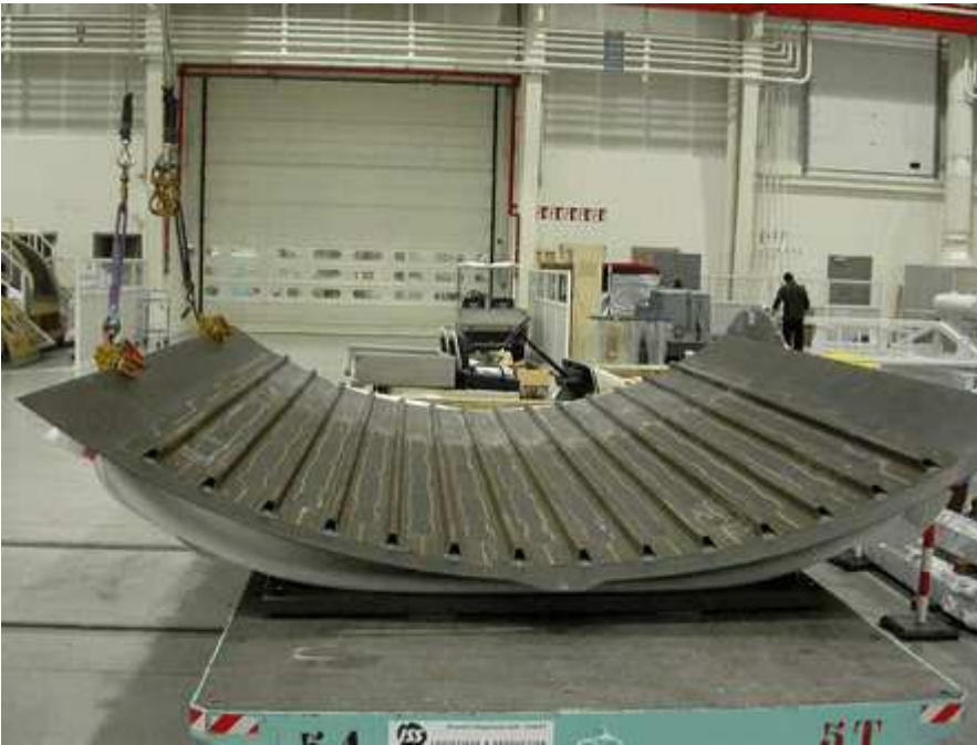
Figure 8.8 Airbus manufactured composite fuselage panels for A350-900 (Flight International, 22/05/08)
