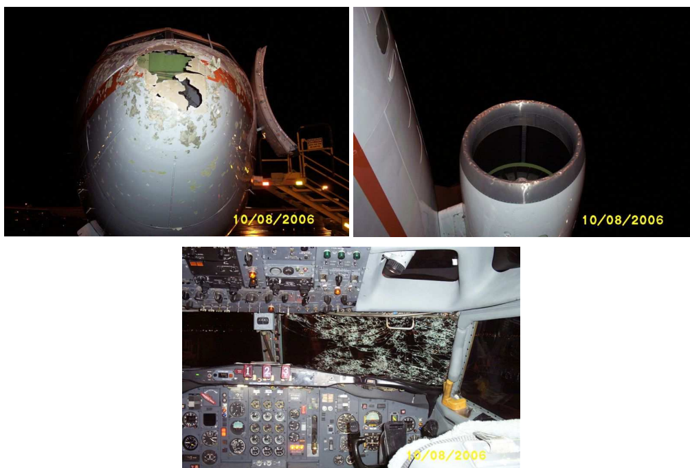
Figure 8.40 Hail damage to BAX aircraft
