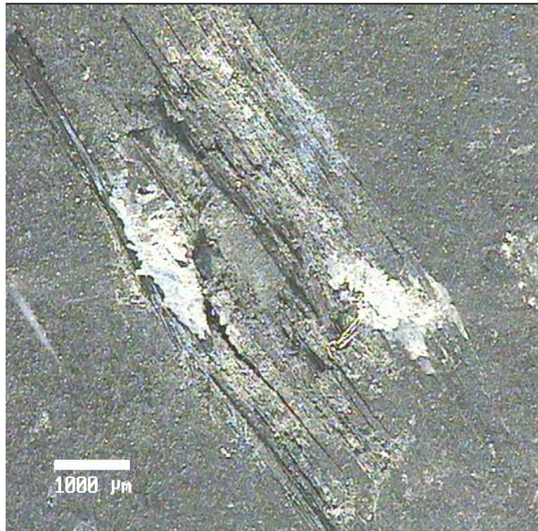
Figure 8.29 Surface damage after impact at increased speeds (from 110m/s to 136m/s)
