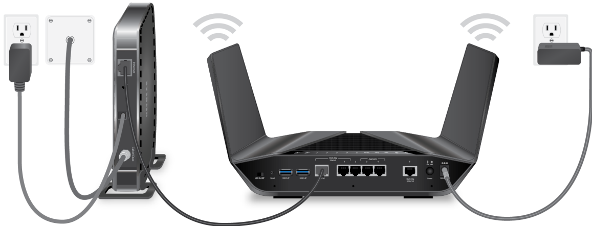
Figure 7. Router connected to a modem
