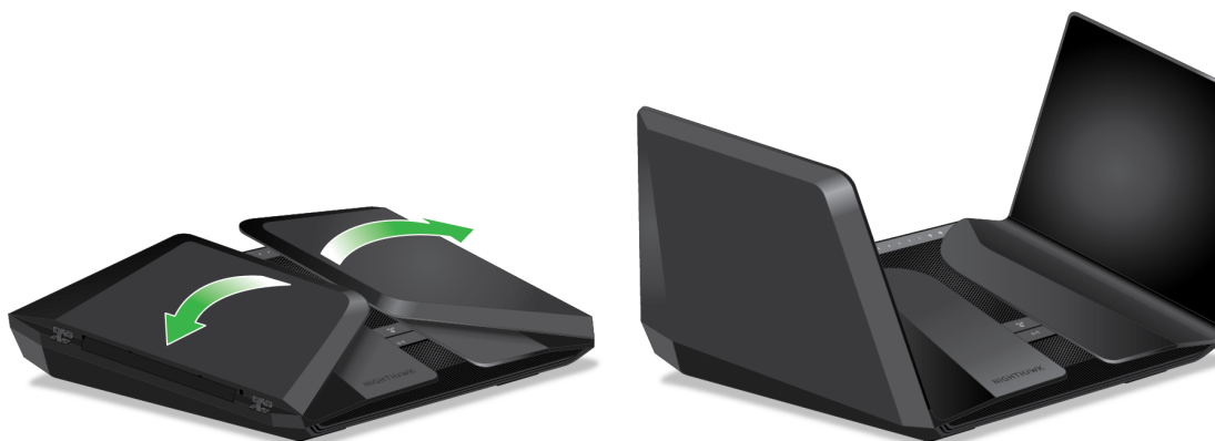
Figure 6. Position the antennas
