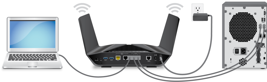
Figure 9. Ethernet port aggregation to a LAN device
