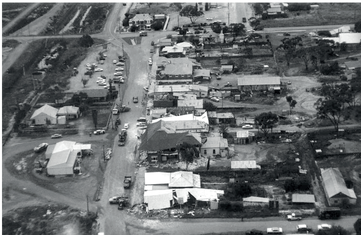
Figure 1. Meckering township immediately after the earthquake on 14 October. Buildings in the foreground and town centre have collapsed and the main street is littered with fallen masonry
