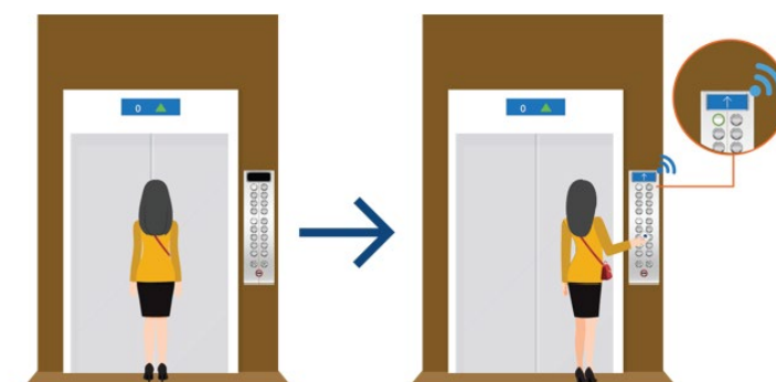
The employee uses their badge again to activate their floor selection in the elevator.
