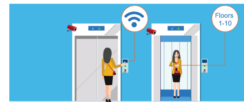
They use their badge to gain access to the elevator assigned to their floor.
