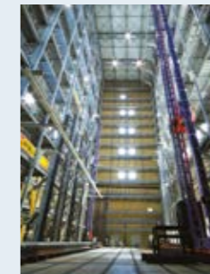
Daifuku's own sway-control technology developed at its high-rise testing tower within the Shiga Works
