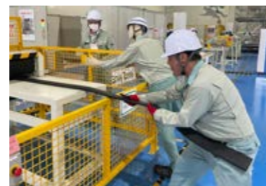
Virtual experience of an accident in which personnel are caught in the roller of a machine
