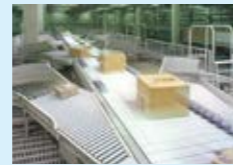
Automated sorters in a distribution center
