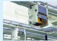
Cleanroom transport systems for semiconductor factory
