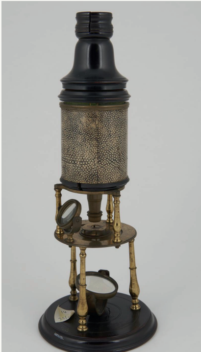
Figure 2: Culpeper microscope with pasteboard body tube and black shagreen support, on flat round base, English, circa 1740. Science Museum Group Collection Online, © The Board of Trustees of the Science Museum. This image is released under a CC BY-NC-SA 4.0 Licence
