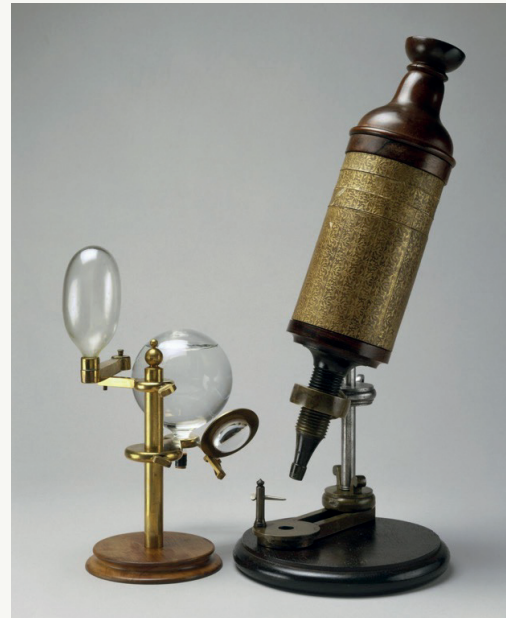
Figure 3: Full size copy of Robert Hooke's original compound microscope. Science Museum Group Collection Online, © The Board of Trustees of the Science Museum. This image is released under a CC BY-NC-SA 4.0 Licence
