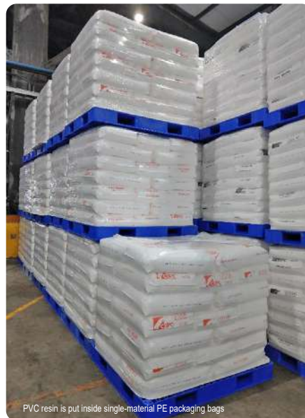
PVC resin is put inside single-material PE packaging bags
