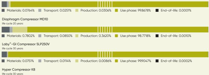
The vast majority of emissions over the entire life cycle of a compressors are caused in the use phase due to the high power range of our compressors, their long lifetime and their uninterrupted operation.
