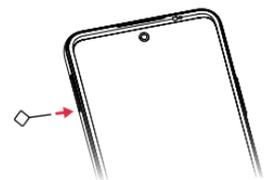
2. Place or remove the Nano SIM card and microSD™ card with the metal contacts facing down into the tray. Gently slide the SIM tray back into the slot.
