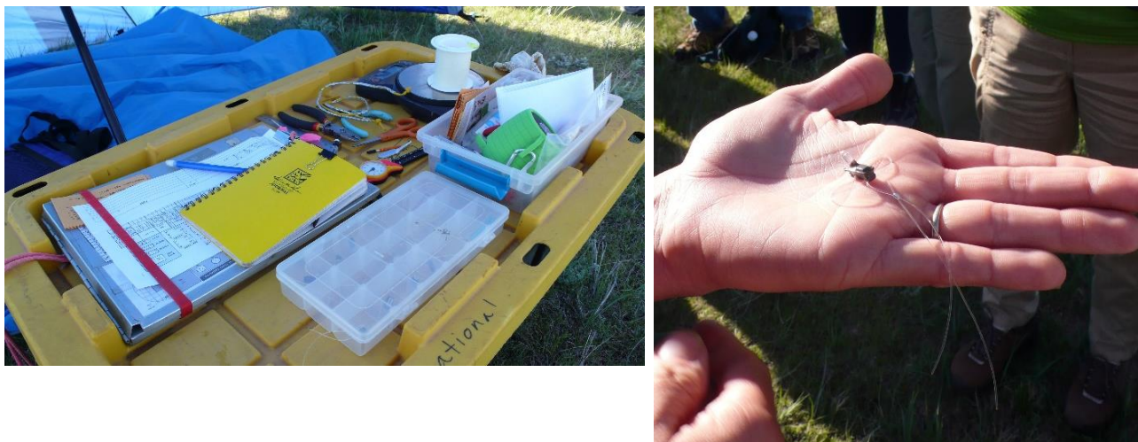
Figure 10: Left - Mobile banding station for attaching geolocators in the field. Right – Geolocator with the beading elastic in the figure-8 loop-leg harness.
