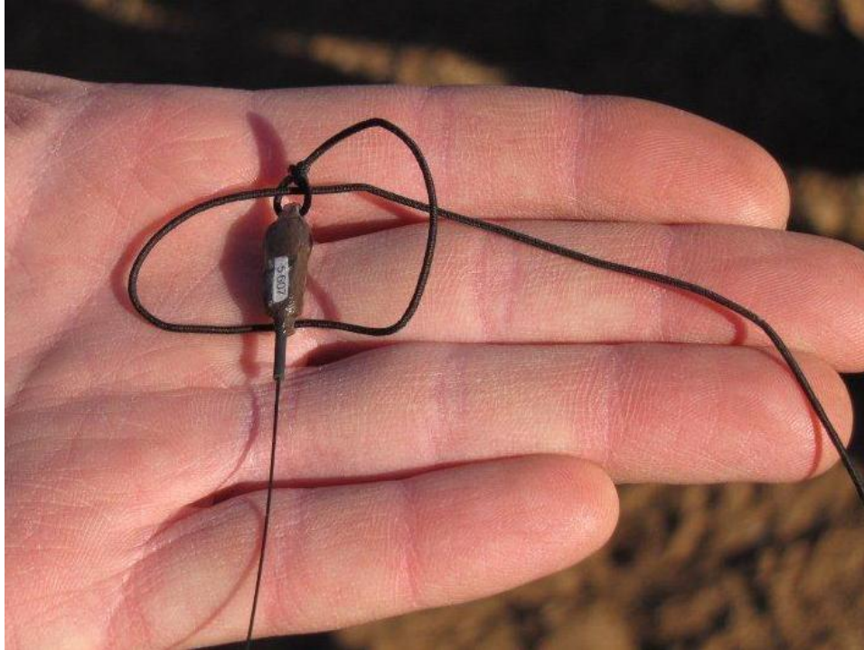
Figure 2. A radio transmitter and harness weighing approximately 0.7 grams. Photograph by Jose Hugo Martinez Guerrero.
