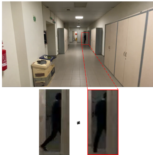
Figure 9: Those shown in the figure are two different people, who however visually appear practically identical. Their appearance descriptor is therefore very similar and this leads the framework to a wrong ID attribution when one of the two leaves the room.
