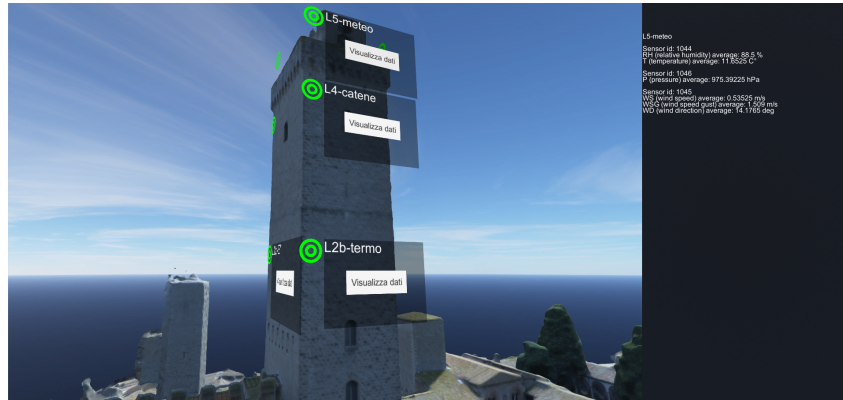
Fig. 3. 3D front end interface. In the main panel, the 3D reconstruction of Torre Grossa in San Gimignano, Italy, can be explored. Installed sensors are gathered from MOSCARDO database and displayed directly. When a sensor is selected, last retrieved data are shown on the right panel.
