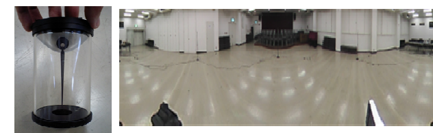
Left: Omni-directional monocular camera. Right: the result of measurement
