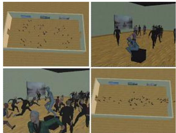
Figure 2: Scenes of simulation of evacuation due to a panic situation. Up-left and up right: before the panic situation, the crowd walks. Down-left and down right: crowd reacts because an event was generated when the statue becomes alive [Musse01].
