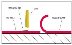
Only once the seam is secure can the second sheet be fitted. To prevent dirt and water from entering seams, seal using a suitable vinyl seaming weld. Silicone sealants can be used around edges where potential for standing water is high, such as in bathrooms.
