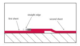
Seams should be stuck using an acrylic adhesive, or double-sided anti-plasticiser tape. Which ever method is applied must be in accordance with the manufacturer's instructions. It is essential that the area being stuck is free from dirt and loose particles. Run a cloth or roller along the seam to flatten the flooring and remove excess adhesive with a damp cloth or white spirit.
