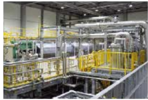
10MW-class alkaline water electrolysis plant
