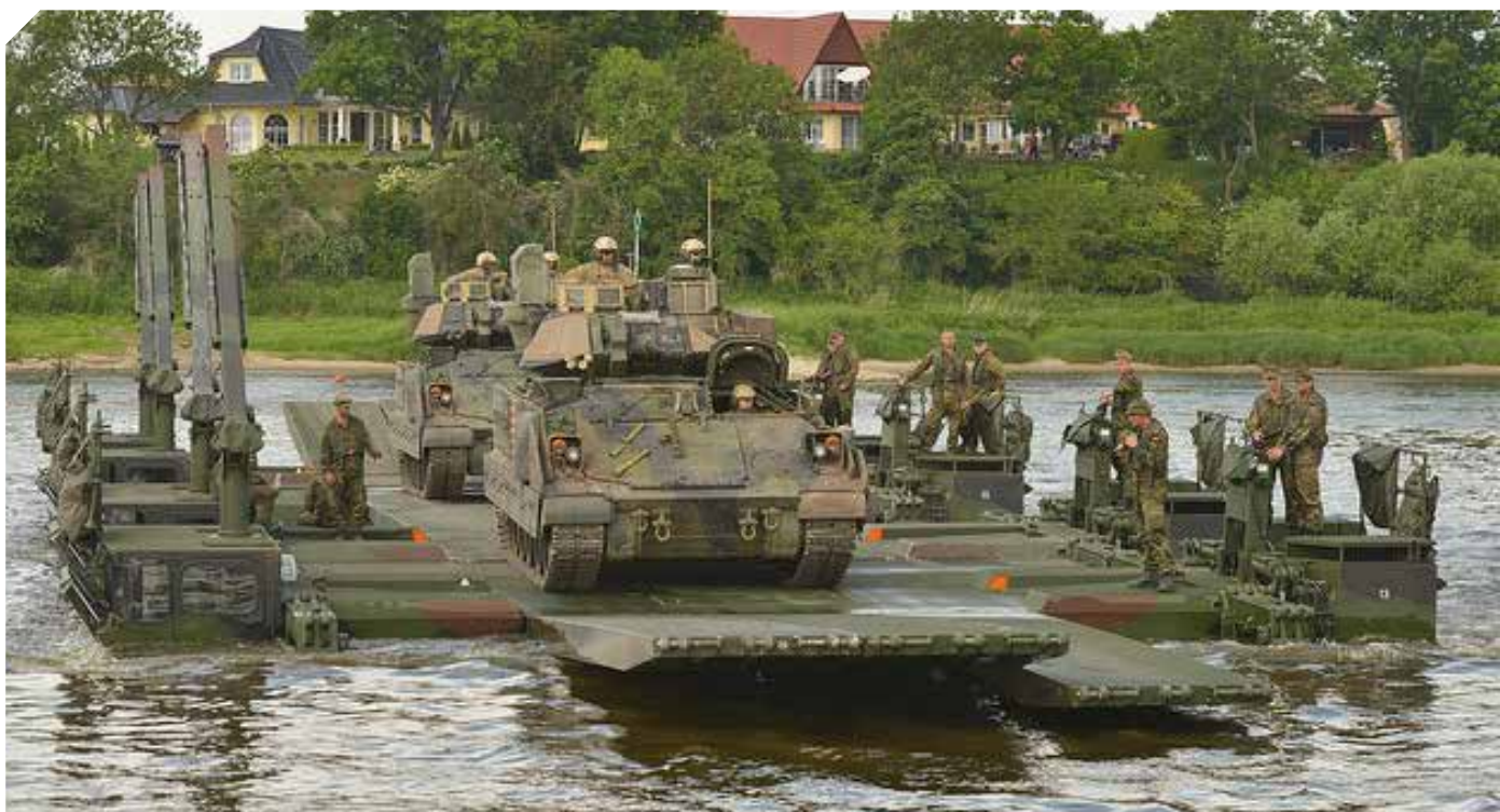
U.S. Army Soldiers, assigned to 1st Armored Brigade Combat Team, 3rd Infantry Division, and German soldiers move M2A3 Bradley Fighting Vehicles during combined river crossing operations at the river Elbe using German army M3 amphibious bridging vehicles during Exercise Heidesturm Shock near Storkau, Germany, June 6, 2015. (U.S. Army photo by SPC Markus Rauchenberger)
