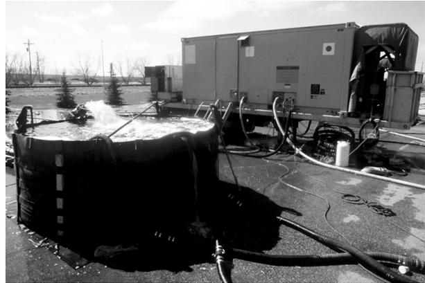
***Reverse Osmosis Water Purification Units provide a reliable way to purify water.***
