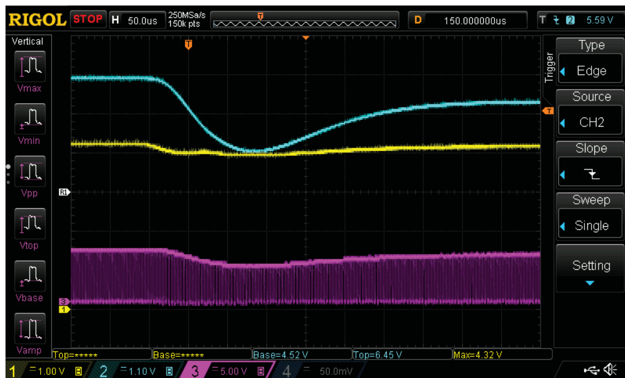
Figure 31: MPPT Operating with a charged super capacitor simulating a battery experiencing a load transient. Load was intense 50mA to 1A transient.
