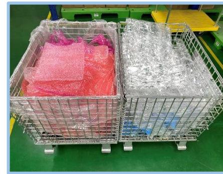
Recycled buffer materials are stored in categories and are retrieved preferentially at the time of shipment.
