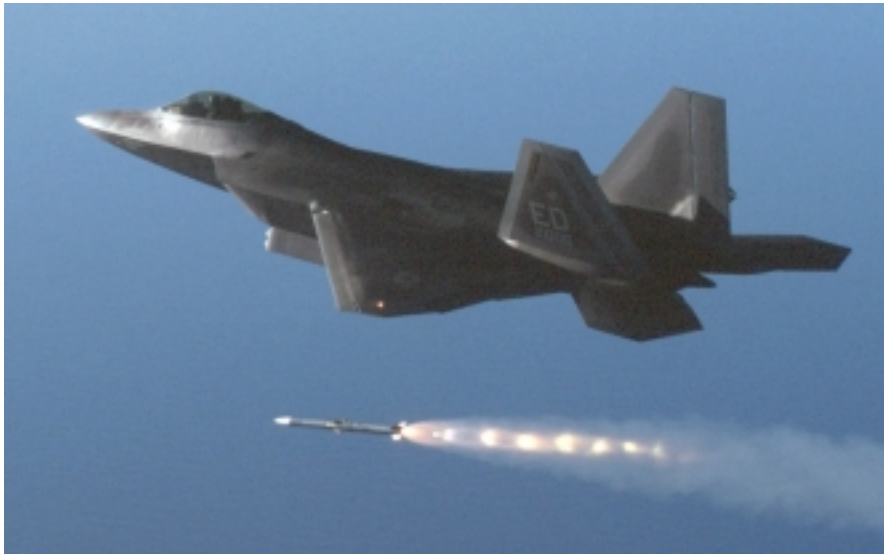
Col. Chris Seat, from Edwards AFB, Calif., fires an Advanced Medium-Range Air-to-Air Missile from an F-22, destroying a subscale drone over a military range in California, in a test of the Raptor's look-down, shoot-down capability.
