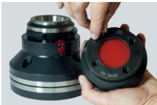
Remove bar seal from housing
