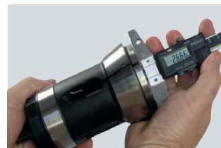
Adjust stopper shaft position
