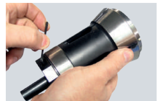
Lock stopper shaft and install
