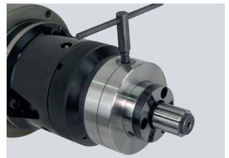
Load a workpiece's internal diameter over the sleeve and actuate the mandrel using the key provided.
