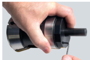
Lock stopper housing in position
