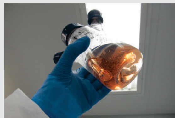
"Spinner" bottle used for the cultivation of neural cells in three dimensions, in this case, brain Organoids
