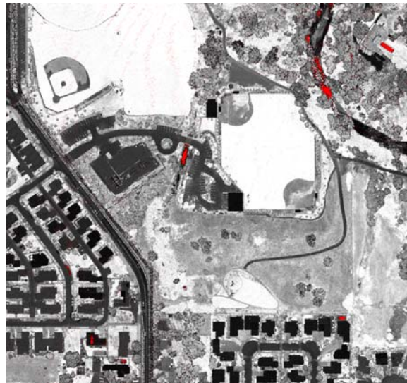
Figure 7. Final image produced using LIDAR intensity data for first returns. Red pixels in the image indicate areas where there were no first returns within the pixel.
