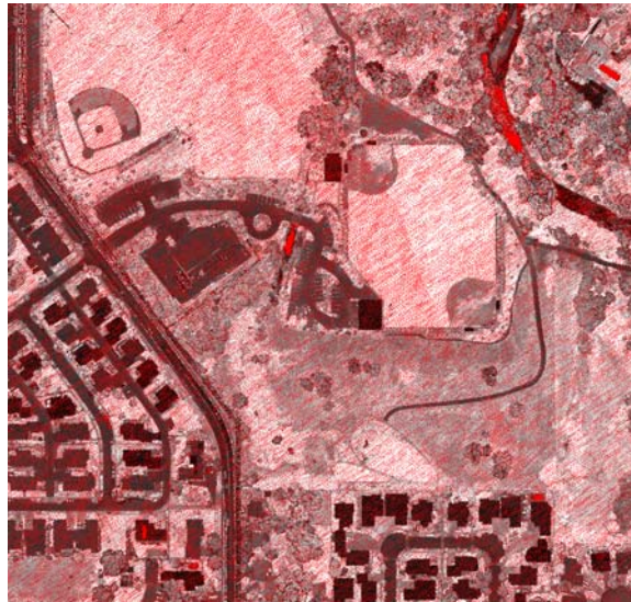
Figure 5. Image produced using LIDAR intensity data for first returns. Red pixels in the image indicate areas where there were no first returns within the pixel. LIDAR data were acquired at a density of 5.5 pulses/m 2 (0.43 m between pulses) using a pulse size of 0.33 m (average diameter at ground level). Image pixels are 0.45 by 0.45 m. Image represents an area that is 434 m wide and 411 m high.
