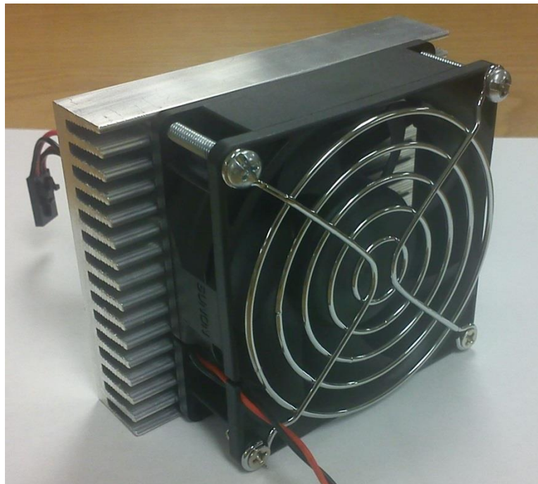
Figure 5.4. Final heat sink and fan assembly.
