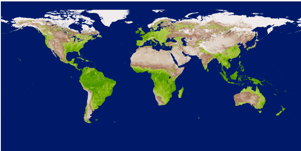
Figure 12: 0.05-deg 16-day MOD13C1 NDVI (upper) and EVI (lower) sample images. The VI values have been pseudo-colored to represent biomass health across the globe using data acquired during April 6-22, 2000.
