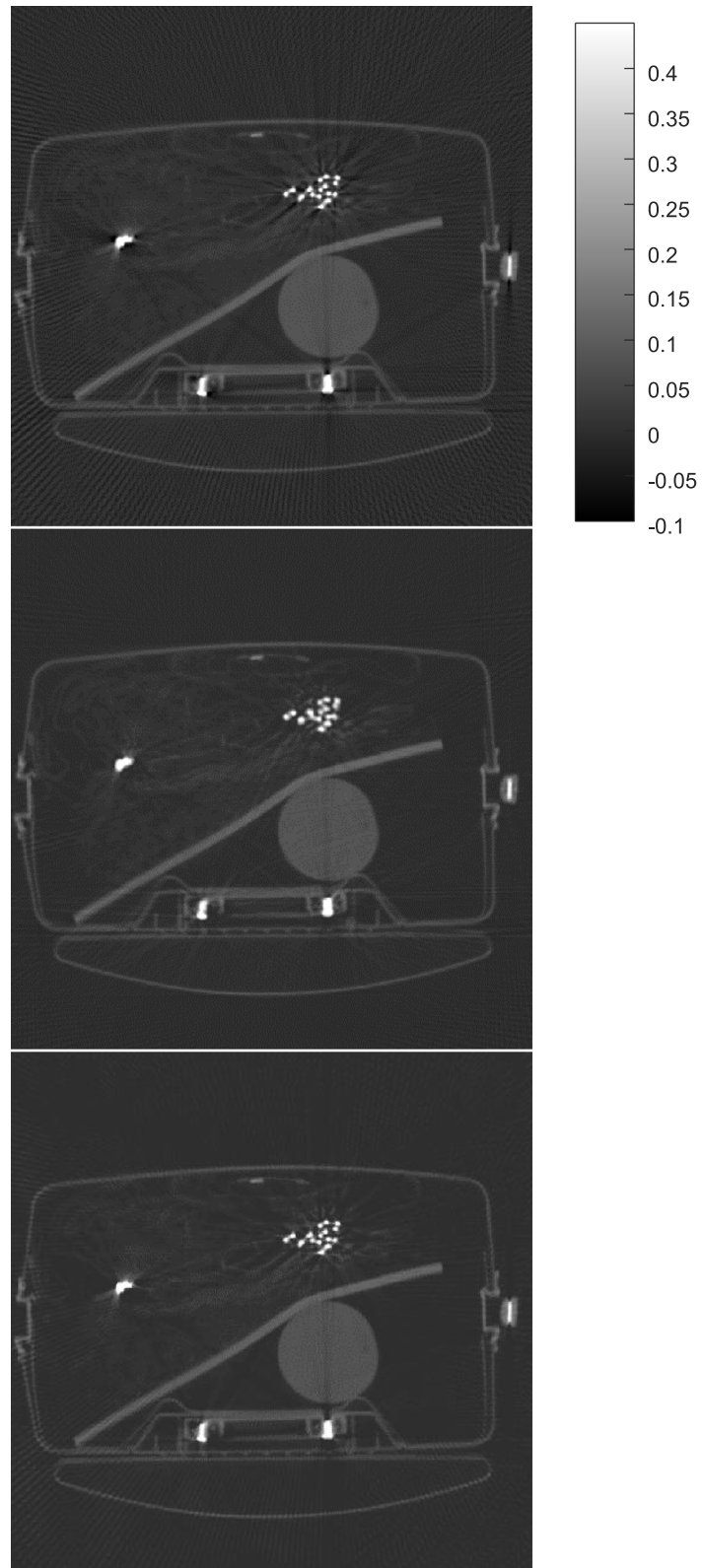
Fig. 1 CT image reconstruction of airport bag #1. Top: the raw FBP reconstruction; Middle: the reconstruction using the proposed algorithm; Bottom: the raw FBP reconstruction with all negative pixel values replaced by zeros
