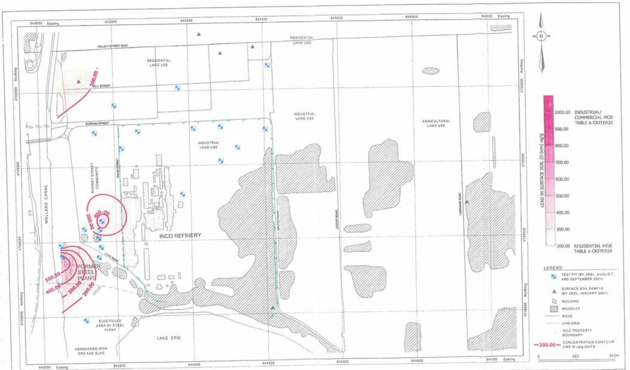
SOIL LEAD CONCENTRATION CONTOURS, 0 TO 5 cm DEPTH EAST SIDE PORT COLBORNE COMMUNITY
