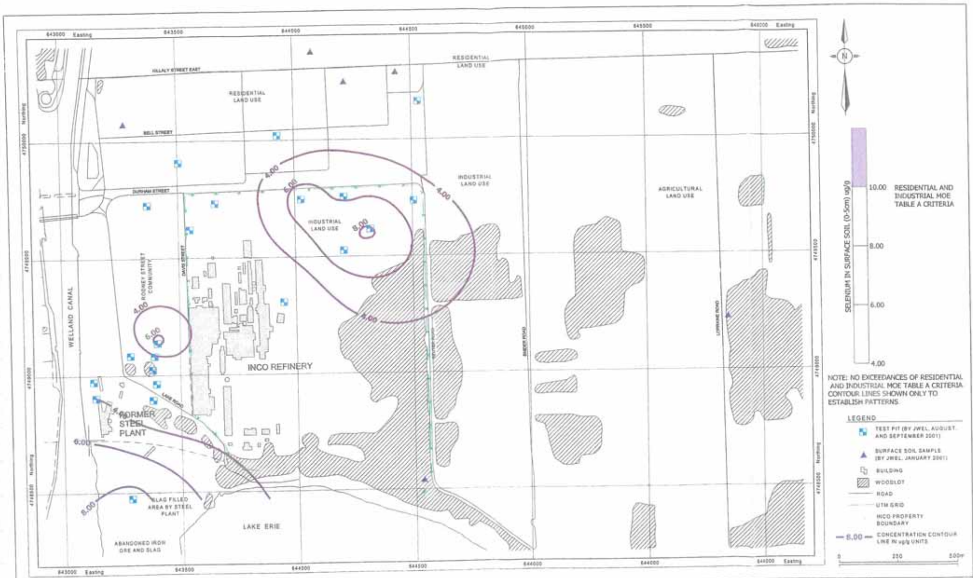
SOIL SELENIUM CONCENTRATION CONTOURS, 0 TO 5 cm DEPTH EAST SIDE PORT COLBORNE COMMUNITY
