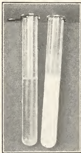
The limewater test. The tube at the right shows the effect of the carbon dioxide.
