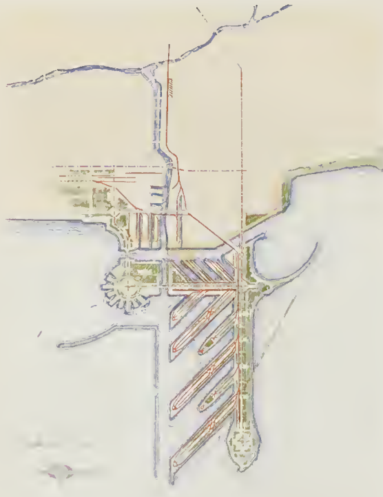
LXXI. CHICAGO. SKETCH DIAGRAM OF DOCKS SUGGESTED AT THE MOUTH OF THE CHICAGO RIVER FOR PACKAGE FREIGHT STEAMERS.
