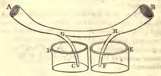
Water propelled into A, passed out at B and C, but not at F. Even if F was immersed in a coloured fluid, this ascended to H, and passed out at B with the water.
