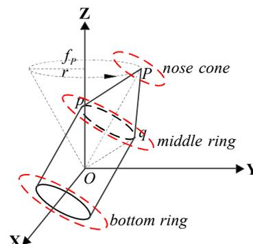
Fig.1. The precession model of ballistic targets
