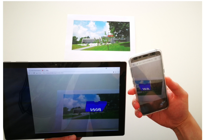
Figure 1: WebAssembly-based natural feature tracking pipeline running on Google Chrome on a Microsoft Surface Pro tablet and a Samsung Galaxy S8 smartphone.
