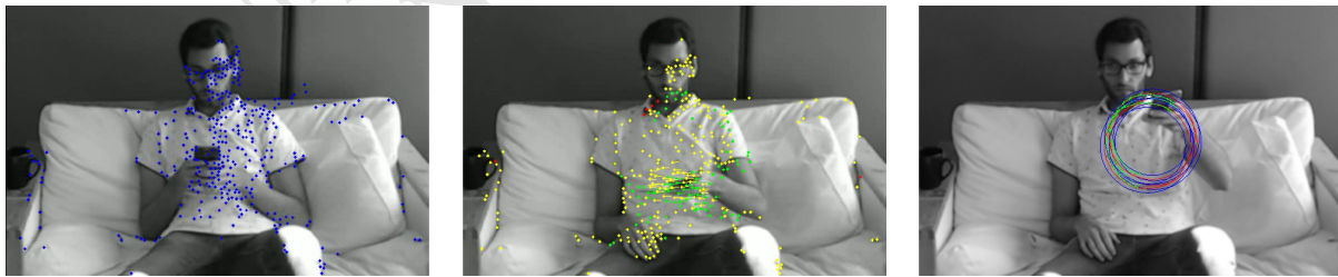
Fig. 2. The stages of TraceMatch for matching the motion of an Orbit using a mobile phone. Left: Features (blue) are detected using the FAST feature detector. Centre: Moving features (green) are compared with the motion of an Orbit using the Pearson correlation. Right: The first feature to be matched is shown with its trajectory (green) and a fitted circle (red) found using RANSAC with inlier thresholds (blue).
