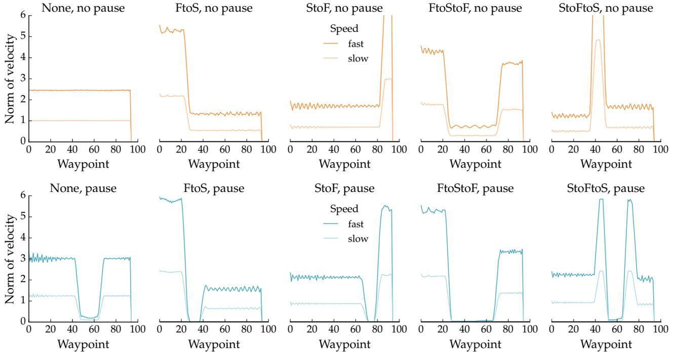
**Figure 2:** Norm of the robot’s configuration space velocity  $v_i$  for each way point configuration  $q_i$  in each of our 20 conditions. Each column is a different speed change pattern, with the top row representing the conditions without a pause and the bottom representing the conditions with a pause, where we see the velocity go to 0. Each plot contains both the slow motion (lighter color) and its fast counterpart (darker color).
