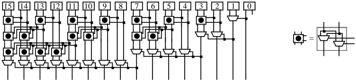
**Figure 5.** The 16 bit Brent-Kung structure. At right is the details of the concatenation block. Note that once the  $Cin$  has been computed for a given stage, a mux is used in place of a concatenation block.
