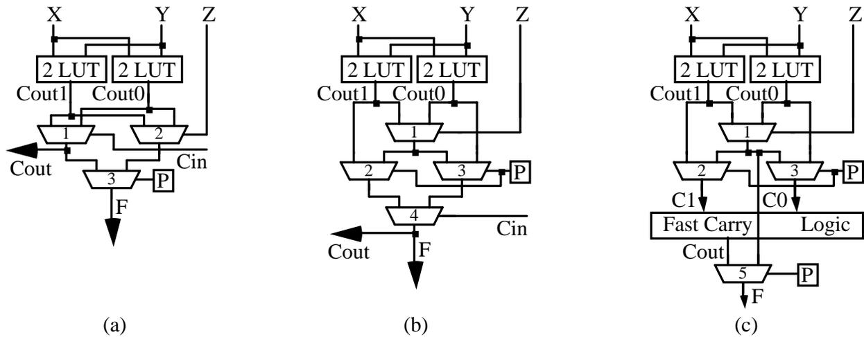
**Figure 2.** Carry computation elements with faster carry propagation.
