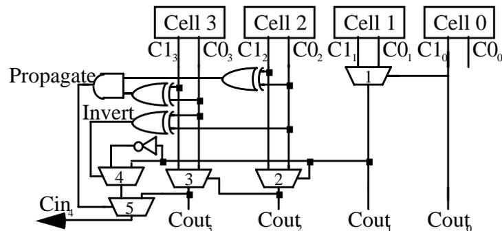
**Figure 4.** The Variable Block carry structure. Mux 1 performs an initial two stage ripple carry. Muxes 2 through 5 form a 2-bit Variable Block block. Mux 5 decides whether the  $C_{in}$  signal should be sent directly to  $C_{out}$ , while mux 4 decides whether to invert the  $C_{in}$  signal or not.
