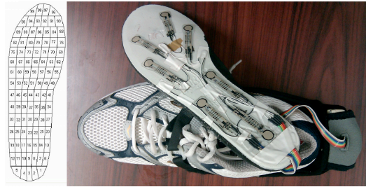
Fig. 1. Right: medical shoe instrumented with pressure sensors. Left: pressure sensor location map under the foot for Pedar's insole. Sensor placement and location are derived from studying Pedar's insole, which has 99 sensors.
