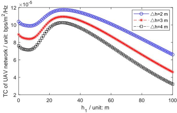
Fig. 6. The relation between the transmission capacity of UAV network user and  $h_1$  with  $\alpha = 0.1$  and different values of  $\Delta h$ .
