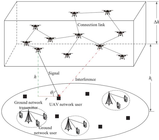
Fig. 1. System model of UAV-ground spectrum sharing.
