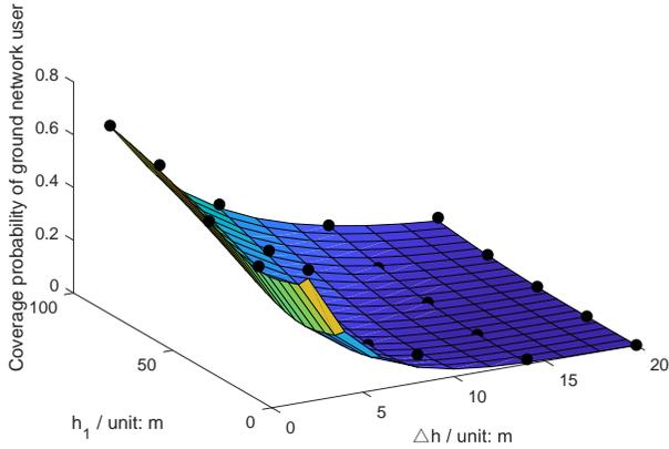
Fig. 2. The coverage probability of ground network user versus  $h_1$  and  $\Delta h$ .
