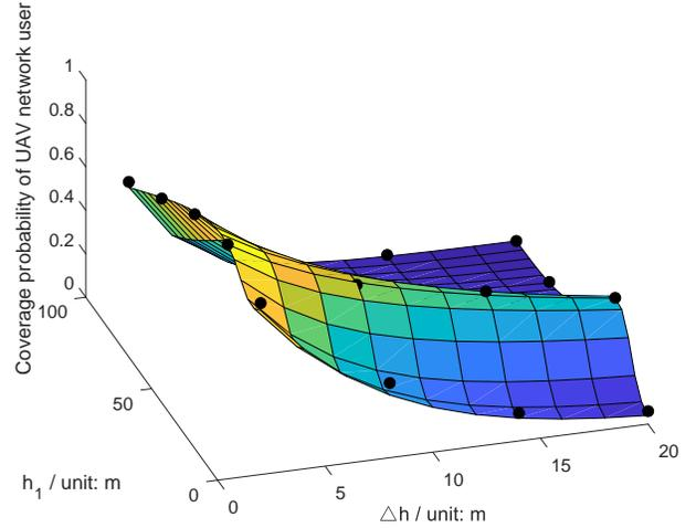
Fig. 4. The coverage probability of UAV network user versus  $h_1$  and  $\Delta h$ .
