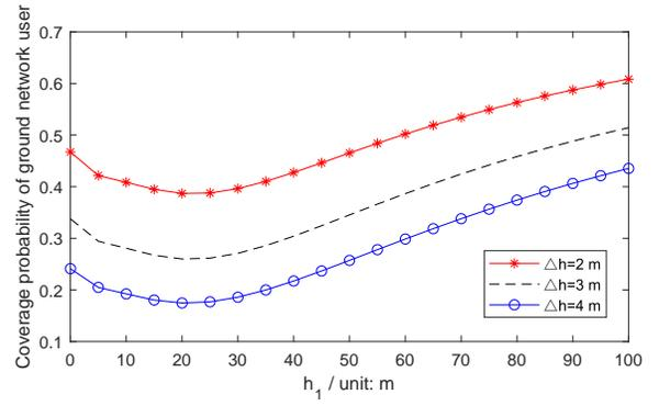
Fig. 3. The relation between the coverage probability of ground network user and  $h_1$  with different values of  $\Delta h$ .
