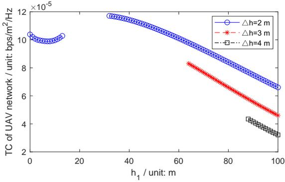
Fig. 5. The relation between the transmission capacity of UAV network user and  $h_1$  with  $\alpha = 0.4$  and different values of  $\Delta h$ .
