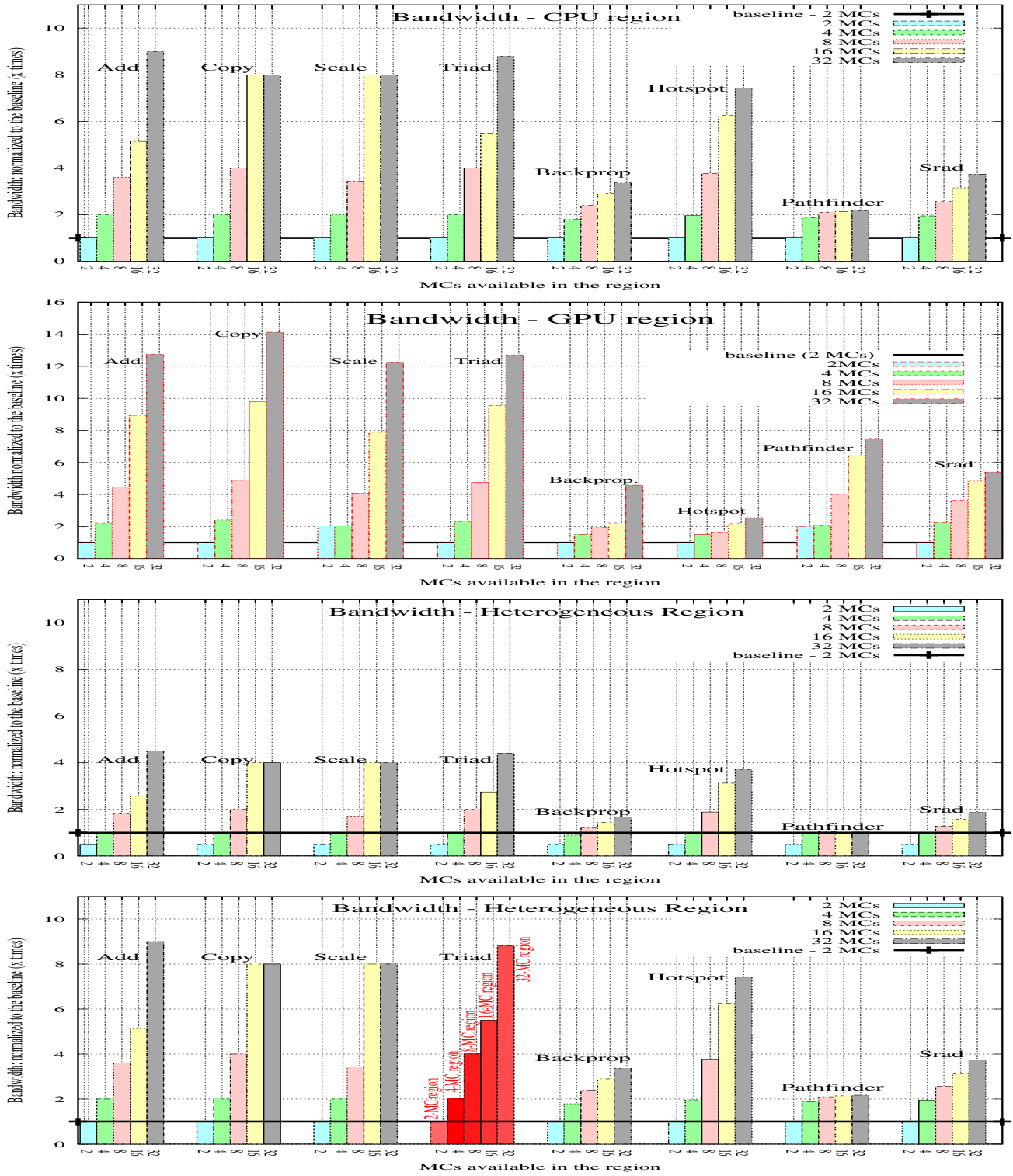
Fig. 3: Fig 3a (top) to Fig 3d (bottom), bandwidth versus number of MCs on Fig 3a for CPU regions, on Fig 3b for GPU regions, and Fig 3c for heterogeneous regions; Fig 3d, reorganization.
