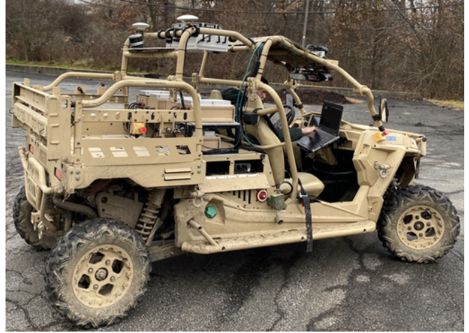
Fig. 15: Off-road test vehicle equipped with a full sensor suite and ROS.
