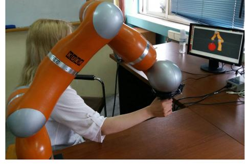
Fig. 3: The user manipulates the master kuka and the slave kuka is simulated in the Rviz.
