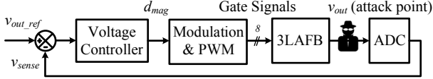
Fig. 2: Block diagram of the constant voltage controller for the 3LAFB. The attacker targets the analog circuitry before the sensing information is digitized by the ADC.
