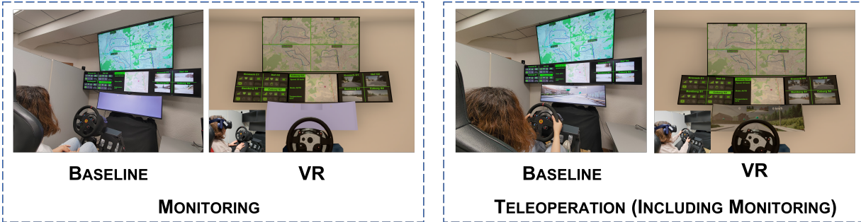
Figure 1: Conditions of Study 1, from left to right: The physical BASELINE interface used in industry in the MONITORING scenario. The replicated VR interface in the MONITORING scenario. The physical BASELINE interface in the TELEOPERATION scenario. The replicated VR interface in the TELEOPERATION scenario.
